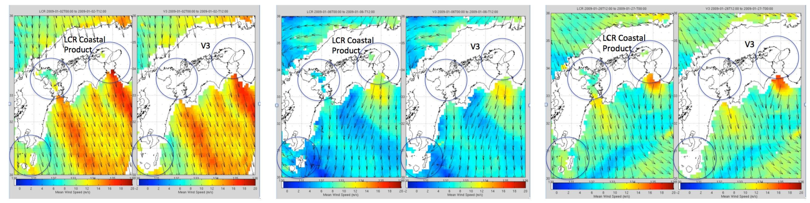
LCRES to LCR comparison: (Southern Japan, Jan 2005), LCRES fills in more vectors near the coast. There are slight differences in the open ocean because the measured rather than theoretical variance is used in wind retrieval. This modification is necessary to account fot residual error variance due to the land contamination correction. The open ocean RMS diifferences vs. ECMWF is similar for both variance formulations. Speed bias needs adjustment for measured variance.
